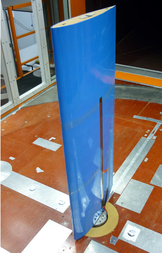
Figure 3.8: Wing in the NWk 1 wind tunnel for preliminary flow control tests with a SDBD plasma actuator mounted on the middle of the three spanwise sections.
