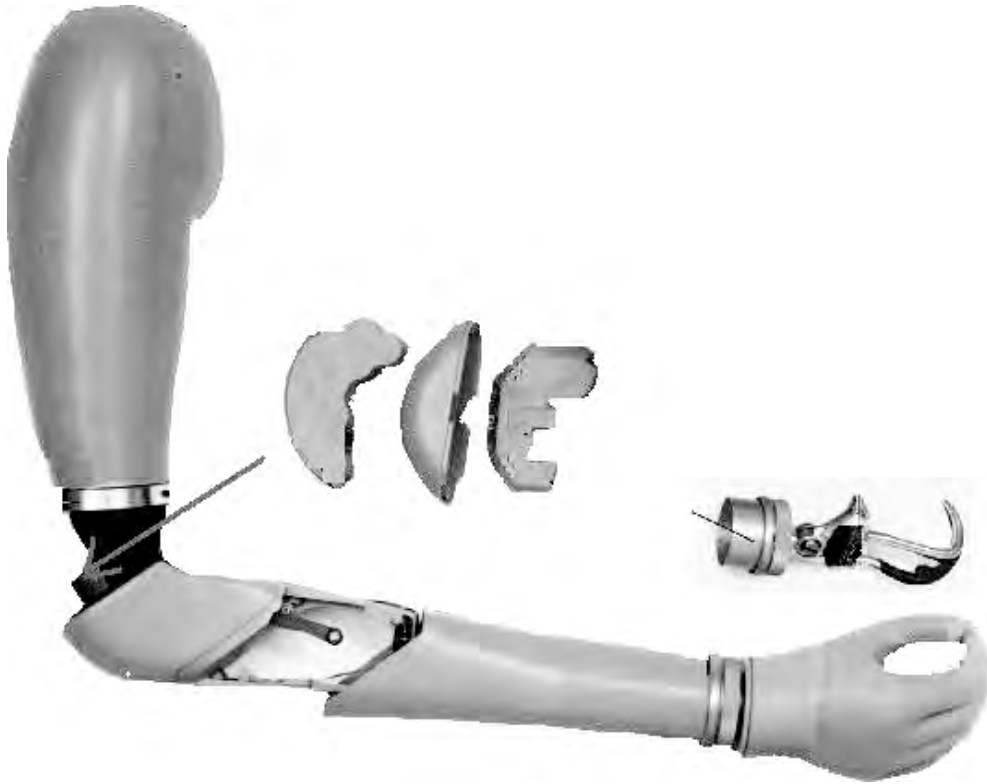
FIGURE 70.6 The Utah arm is a self-contained battery powered artificial arm–hand complex. The system comprises myoelectric control of the elbow, wrist, and grasping movements.
