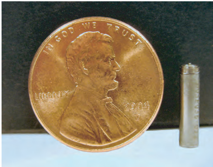
FIGURE 34.2 Quallion battery for the BPB.
