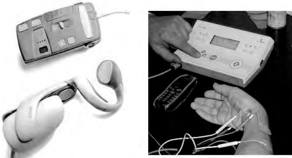
FIGURE 70.1 Handmaster NMS1 (NESS, Israel) grasping device for tetraplegic and hemiplegic patients (left). Actigrip CS (Neurodan A/S, Denmark) is the surface functional electrical therapy system (right). (See text for details.)
