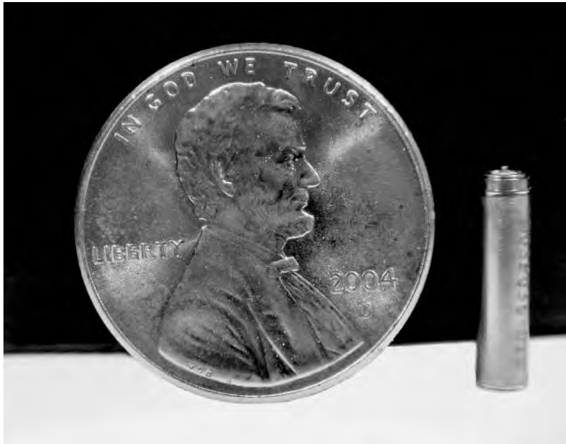
FIGURE 34.2 (See color insert following page 32-14.) Quallion battery for the BPB.
