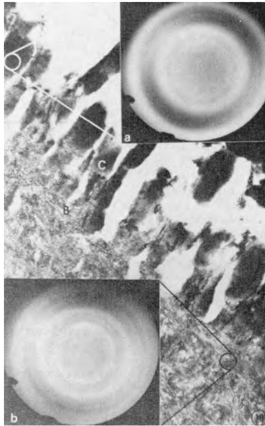
FIGURE 39.15 Transmission electron micrograph of well-mineralized bone (b) juxtaposed to the glass-ceramic (c) which fractured during sectioning. \times 51,500 . Insert a is the diffraction pattern from ceramic area and b is from bone area. (From Beckham C.A., Greenlee T.K. Jr, and Crebo A.R. 1971. Calc. Tiss. Res. 8: 165–171. With permission.)
