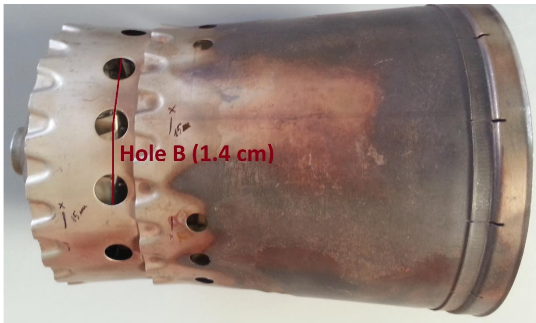
Figure 3.6 Layout of liner injection holes B
