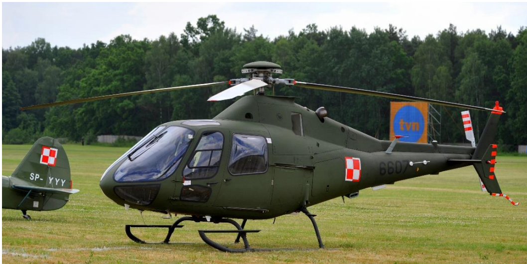
Figure 1.1 Helicopter model PZL SW-4 RR250C20R2 [4]
